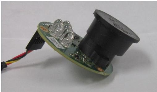
**Figure 30: LeddarOne™ with Light Shielding Installed on its Lens**
