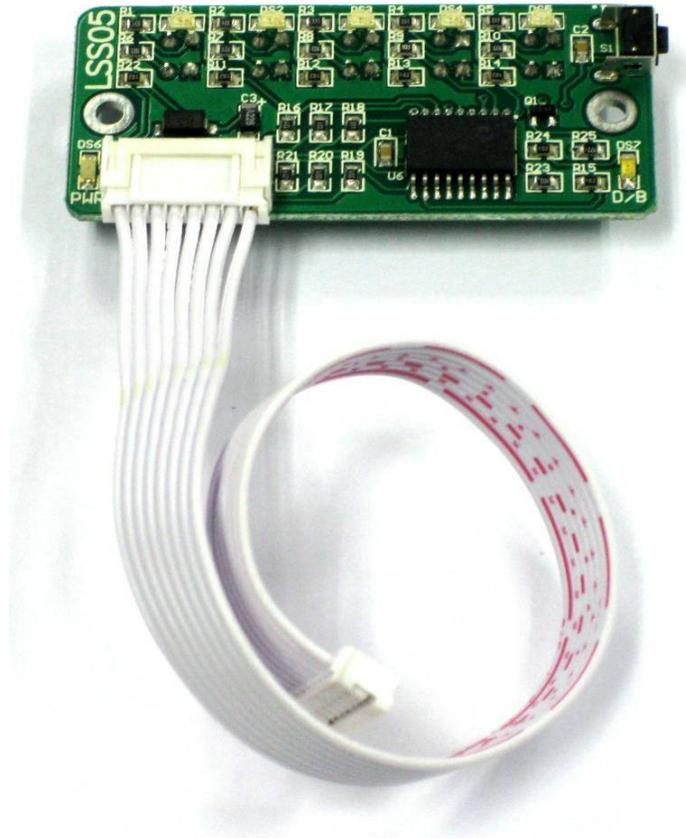
1. LSS05 PCB with every component soldered properly.
