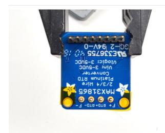
Solder in both pins of each terminal block. You can remove the tape when done.
