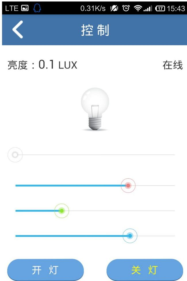
In this interface, you can switch to test the LED lamp on the board , can also control the brightness of the LED red, green and blue three lights by dragging the panel .And The test panel brightness data can be displayed on the upper left corner of the APP!
