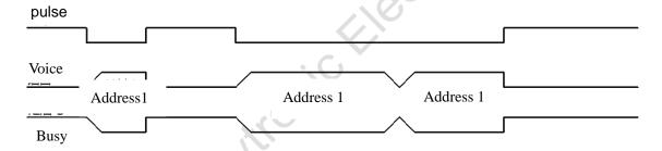
Note: High level stops when I / O port are low level and keep play. Continue to keep a low level even if the first time is over. It will go along replay until change into high level. Low level has sound. High level doesn't have.
