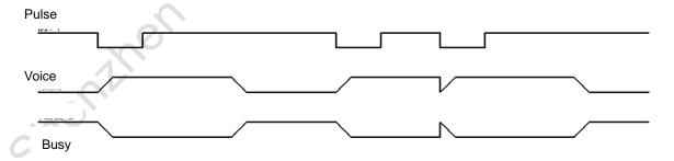
Note: Negative trigger pulse. When I / O port inspects the falling edge (for example, I / O port click short-circuit to GND more than 25ms), Voice will be broadcast. If do that again, Voice are still playing, it will be interrupted and replay. Therefore, it will be replay as long as has falling edge signal.
