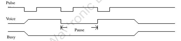
Note: Negative trigger pulse. The first pulse (for example, I / O port click short-circuit to GND more than 25ms) voice is playing but in a suspended state. The second pulse still working, which triggers the suspension of the voice. BUSY remain in this state.
