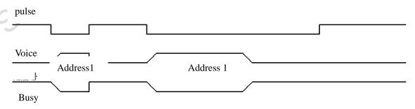
Note: Trigger level. High level stops when I / O port are low and keep play. It will be not continue to play even if the first time is over and keep a low level. The voice just plays one time after being triggered.
