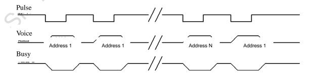
Note: Negative trigger pulse. Trigger with a key to play a sound (for example, I / O port click short-circuit to GND more than 25ms). A pulse plays a piece; the next pulse plays the next piece. Repeat
