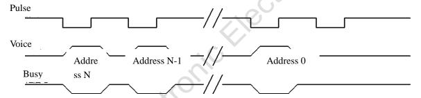
Note: Negative trigger pulse. Trigger with a key to play a sound (for example, I / O port click short-circuit to GND more than 25ms). A pulse plays a piece; the next pulse plays the last piece. No longer trigger forward when the front voice is over. Repeat the operation; it only can play to the last.
