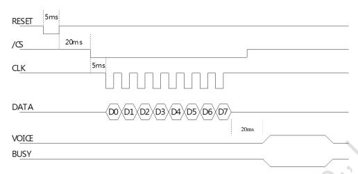
Note:Reset signal is only used in the environment of the external disturbance is strong, if not special industrial occasions, do not need to send the reset signal, can be sent directly to select-chip(cs), the clock(clk) and data signals.
