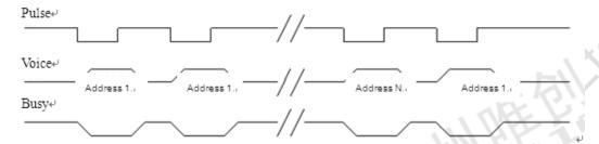
Note: Negative trigger pulse. Trigger with a key to play a sound (for example, I / O port click short-circuit to GND more than 25ms). A pulse plays a piece; the next pulse plays the next piece. Repeat the operation. It will start again from the first piece when the last shows off. Loop continuously.
