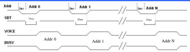
During the triggering process, the stable time of address signal is 5ms, then the SBT can be sent to trigger the voice play after the address is sent 5ms later, and the maintenance time of SBT trigger is 25ms. When sending SBT continuously, ensure that the interval between two address commands is more than 85ms.
