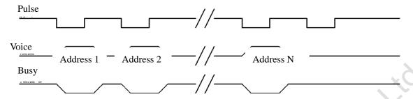
Note: Negative trigger pulse. Trigger with a key to play a sound(for example, I / O port click short-circuit to GND more than 25ms). A pulse plays a piece, the next pulse plays the next piece. It doesn't stop until the last piece is finished. Repeat the same operation. It only can play to the last.
