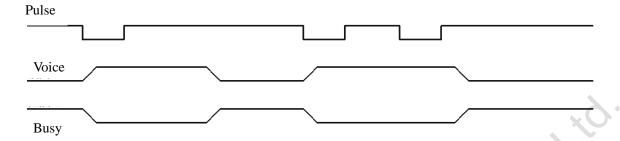
Note: Negative trigger pulse. When I / O port inspects the falling edge (for example, I / O port click short-circuit to GND more than 25ms), Voice will be broadcast. If do that again during playing, the voice will not be interrupted and continue to broadcast. To be valid unless the voice at an end and inspects the falling edge.
