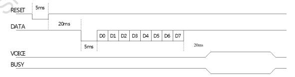
RESET is the RESET signal, and the chip is RESET before the data is sent. If it is not in a special industrial
