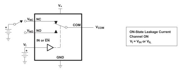
Figure 19. ON-State Leakage Current (I<sub>COM(ON)</sub>, I<sub>NC(ON)</sub>)
