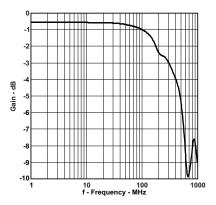
Figure 29. Gain vs Frequency Bandwidth ( $V_{+} = 1.8 V$ )
