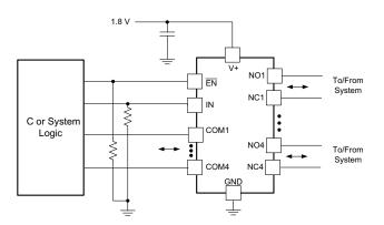
Figure 28. System Schematic for TS3A5018
