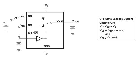
Figure 18. OFF-State Leakage Current (I<sub>COM(OFF)</sub>, I<sub>NC(OFF)</sub>, I<sub>NO(OFF)</sub>)
