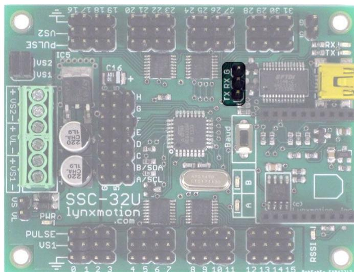
The three pins behind the FTDI chip are Tx, Rx and GND. Commands sent from the SSC-32U are done using the Tx pin while commands to be received by the SSC-32U are done via the Rx pin. These pins allow you to easily send commands to the servo controller from another microcontroller. To do so, connect the Tx pin on the microcontroller to the Rx pin on the SSC-32U, the Rx pin on the microcontroller to the Tx pin on the SSC-32 and GND to GND.
