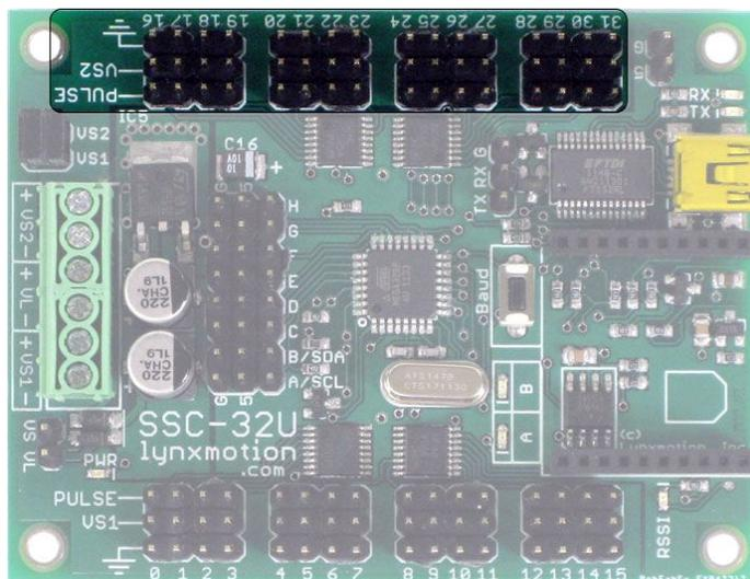
This is the second set of 16 pins. Pins 16 to 31 correspond to VS2. The outermost pin (farthest from the center of the board) is the ground pin (normally the black wire in a three pin cable). The center pin corresponds to the voltage (normally the red wire) and is marked with VS1. The last pin is the signal pin which sends the position command to the servo. The signal wire's color may vary, but is normally white or yellow.
