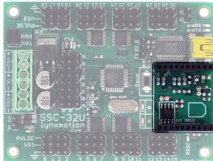
The XBee headers allow you to connect an XBee wireless module or other XBee compatible devices. Take note of the image on the board for how to orient the module. Please refer to the communication / control section in this guide for more information.
