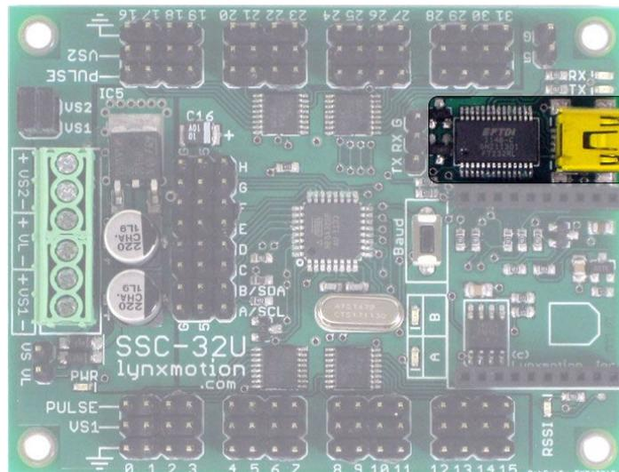
Commands can be sent to the SSC-32U's microprocessor from the computer via the onboard USB port. The microprocessor can only understand commands sent in serial (not USB) format, so an FTDI chip (the area highlighted next to the USB port) converts the USB datastream to serial and allows the board to be picked up by your computer's COM port once connected. Please refer to the drivers section below for more information.
