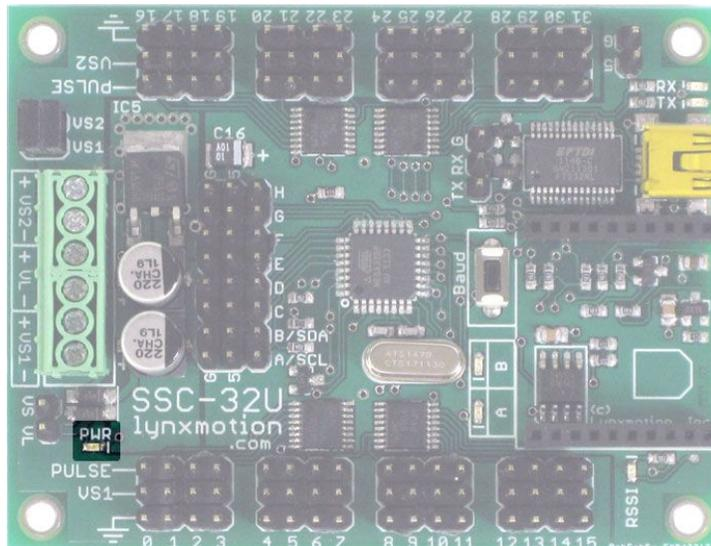
The PWR LED is connected to V\_logic which is the equivalent of  $\text{MAX}(V_L, VS1)$  minus roughly 0.7V. It's the voltage that's then regulated to 5V for powering the logic circuits. The LED is lit when the microcontroller onboard receives adequate power.
