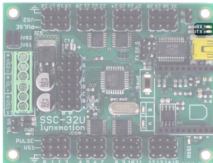
The two LEDs next to the USB port provide the user with visual feedback of when data is received (Rx) and if data is transmitted (Tx). These are only associated with communication via the USB port and not the XBee header or serial pins.
