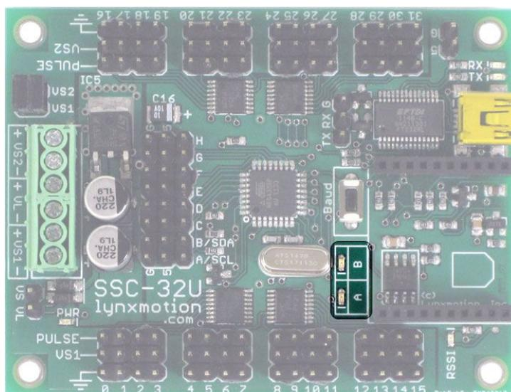
There are two distinct LEDs on the board labeled A and B. When not setting the Baud rate, the LEDs indicate the following:
