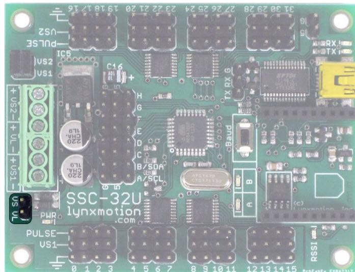
These two pins allow you to tie the VS1 terminal to VL (i.e.  $VL = VS$ ). This would have the same effect as running a wire from from the VS1+ screw terminal to the VL+ screw terminal. Please refer to the power section of this guide for important information. A jumper for these pins is not included.
