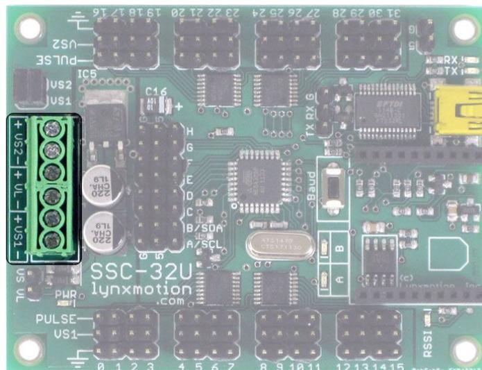
VS1 provides power directly to pins 0 to 15 (ideally 4.8V to 6V for standard RC servos)
