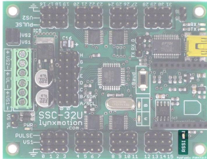
RSSI stands for “Received Signal Strength Indication” and the LED is connected to pin 6 of the Xbee socket. Different blink intervals are used to indicate different status based on the module chosen.
