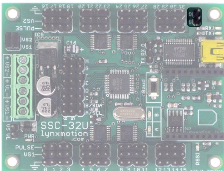
These pins are normally not needed, and pins are not provided. Should the two capacitors onboard not be sufficient for your application, a third capacitor can be added here. If you are not well versed in electronics, we suggest not touching this part of the board.
