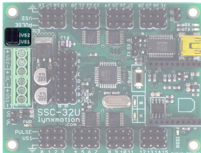
These 2x2 pins allow you to set  $VS1 = VS2$ . This would have the same effect as running a wire from the VS1+ screw terminal to the VS2+ screw terminal. There are two jumpers to handle higher current. The board is shipped with these in place and it is up to the user to remove them if needed. Please refer to the power section of this guide for important information.
