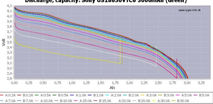
Discharge, capacity: Sony US18650VTC6 3000mAh (Green)
