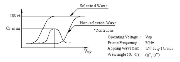
Contrast ratio(Cr) =  $\frac{Brightness \ of \ selected \ dots}{Brightness \ of \ non-selected \ dots}$
