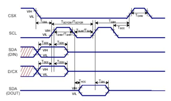
6.5 i80-System Interface Timing Characteristics
