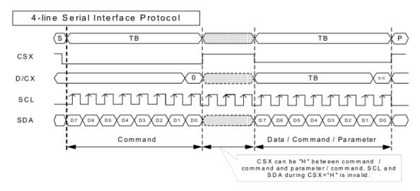
Figure6: 4-pins Serial Protocol for writing register or GRAM
