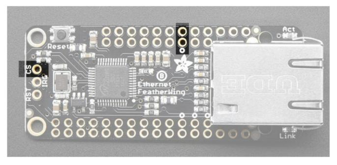
Which is connected to pin**#10** on Feather Teensy 3, 32u4 and M0, pin**#15** on ESP8266, and **PB4** on WICED.
