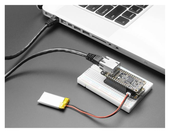
Each order comes with one assembled and tested FeatherWing, plus some header. You will need to solder in the header yourself but its a quick task.
