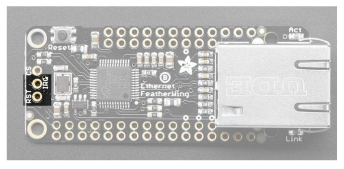
You can also connect to and use the**IRQ** and WIZ **ReSeT** pins. These are not used in the library and are there for advanced usage. They are 3.3V logic, 5V tolerant.
