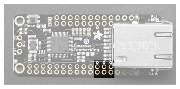
Configuration, setup, and data is received/transmitted over SPI. All Feathers have the default SPI port on the same pins, so we use **MOSI/MISO/SCK** in this location. They are 3.3V logic, 5V tolerant.
