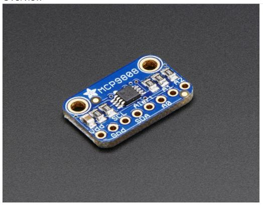
This I2C digital temperature sensor is one of the more accurate/precise we've ever seen, with a typical accuracy of  $\pm 0.25$ °C over the sensor's -40°C to +125°C range and precision of +0.0625°C. They work great with any microcontroller using standard i2c. There are 3 address pins so you can connect up to 8 to a single I2C bus without address collisions. Best of all, a wide voltage range makes is usable with 2.7V to 5.5V logic!
