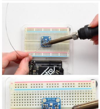
And Solder! Be sure to solder all pins for reliable electrical contact.
