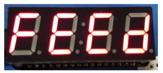
You can also adjust the brightness and blinking of the 7-segment display just like with the matrix display above. See the matrix brightness and blinking section for details on the functions to call.
