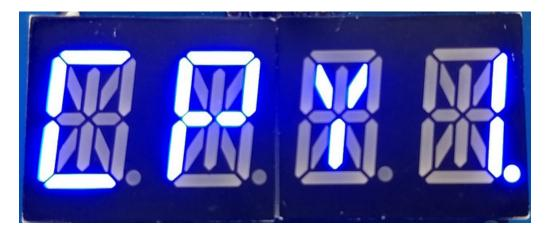
And just like with the 7-segment display you can use the brightness and blink functions just like with the matrices to control those attributes of the display!
