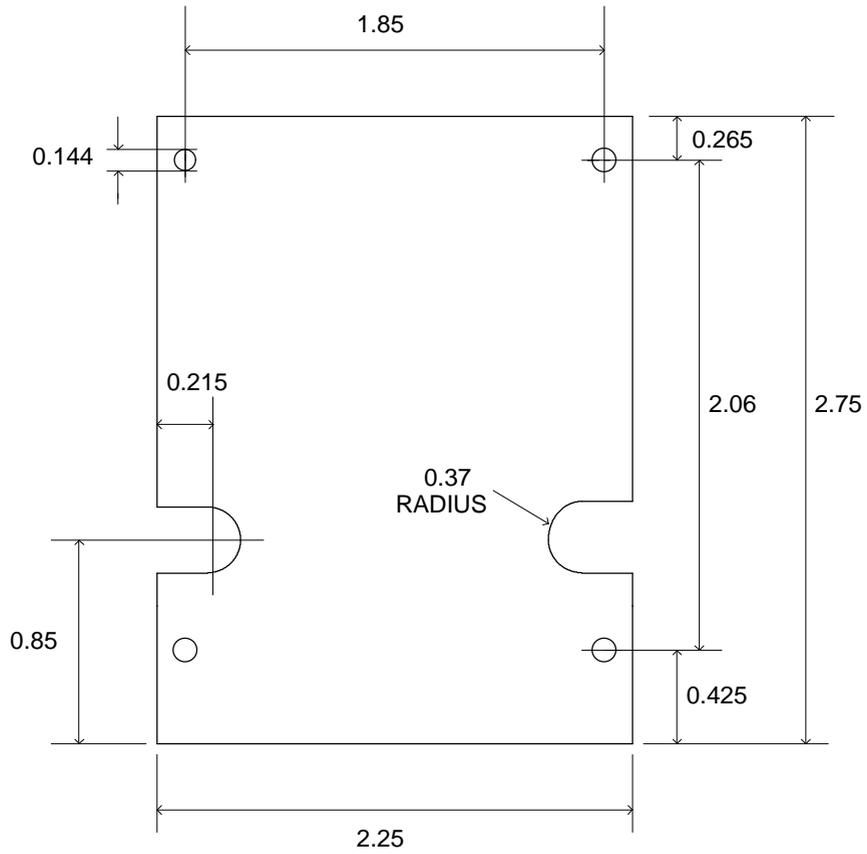
DIMENSIONS OF PRINTED CIRCUIT BOARD
