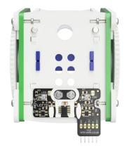
**Examples of board in use:** This breakout board can be used with our :MOVE mini robot. For more details see: <a href="www.kitronik.co.uk/movemini">www.kitronik.co.uk/movemini</a>
