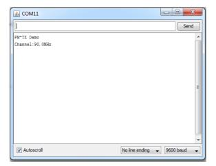
Then you could input data through Serial Monitor to change the frequency. To change the frequency to 85.0MHZ, I send &0850:
