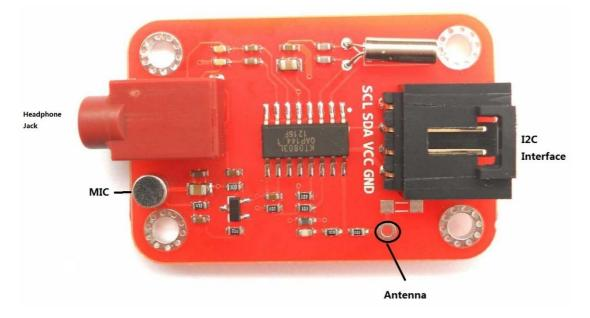
The anti-reverse 4pin header is I2C interface. And the headphone jack is the red one, through which you could input the audio signal. Beside the jack, there is a small MIC. You could speak to it and your voice will be modulated on FM radio.
