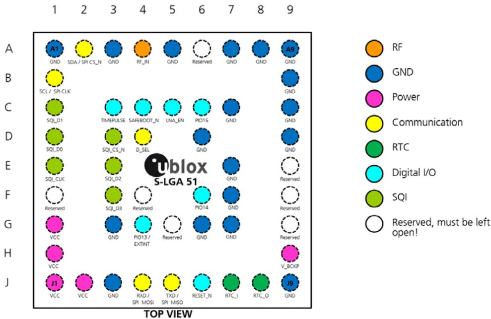
Figure 2: Pin assignment of ZOE-M8G (S-LGA51), top view
