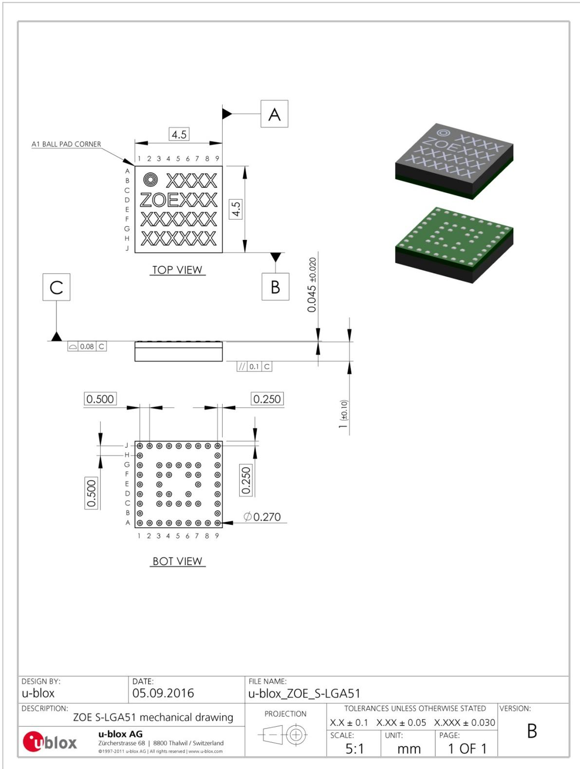
Figure 5: Mechanical drawing for ZOE-M8 (S-LGA), bottom view
