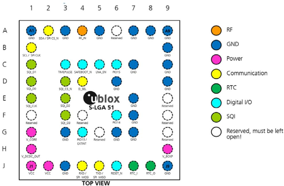
Figure 3: Pin assignment of ZOE-M8Q (S-LGA51), top view
