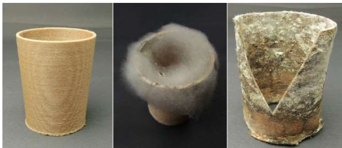
left: fresh printed GROWLAYbrown middle: cotton-like mold growth right: slow-growing lichen
