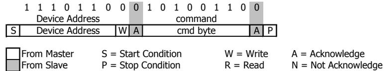
Figure 6: I<sup>2</sup>C Command to read memory address= 011
