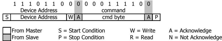
Figure 5: I<sup>2</sup>C Reset Command
