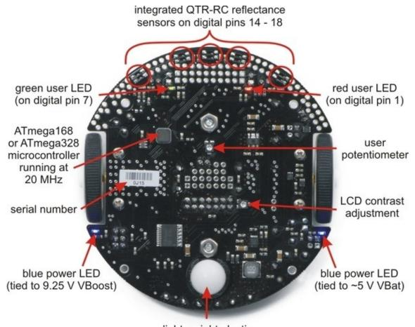
light-weight plastic ball caster Labeled bottom view of the Pololu 3pi robot.
