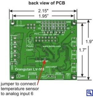
Orangutan LV-168 bottom view with dimensions (Arduino pin mapping).
