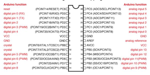
Digital Pins 11,12 & 13 are used by the ICSP header for MISO, MOSI, SCK connections (Atmega168 pins 17,18 & 19). Avoid low-impedance loads on these pins when using the ICSP header.
