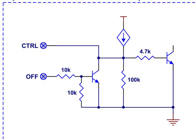
Input structure of ON input
