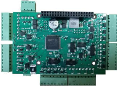
The second generation of our Industrial Automation card brings to the Raspberry Pi platform all the building blocks required for Industrial Automation projects. Stackable to 8 levels, the card works with all Raspberry Pi versions, from Zero to 4.
