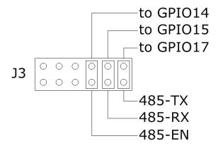
If jumpers are installed, Raspberry Pi can communicate with any device with an RS485 interface. In this configuration the MEGA-BAS card is a passive bridge which implements only the hardware levels required by the RS485 protocol. To use this configuration, you need to tell the local processor to release control of the RS485 bus:
