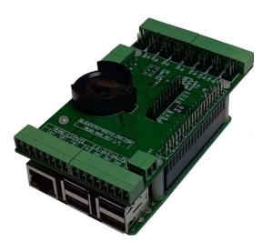
The second generation of our Building Automation card brings to the Raspberry Pi platform all the building blocks required for Building Automation projects. Stackable to 8 levels, the card works with all Raspberry Pi versions, from Zero to 4.
