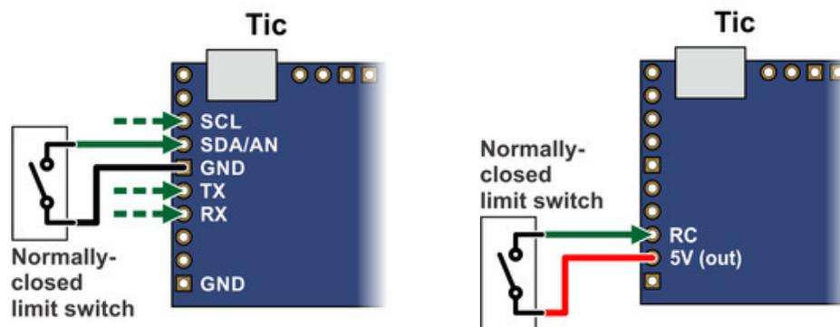
Once you have configured and connected the limit switches, you can test them. Connect the Tic to USB and activate the limit switches (e.g. press them with your hands) while looking at the “Limit switches active” field in the “Status” tab. By default, it should say “None”. When you activate a limit switch, the field should indicate which limit switch direction has been activated.
