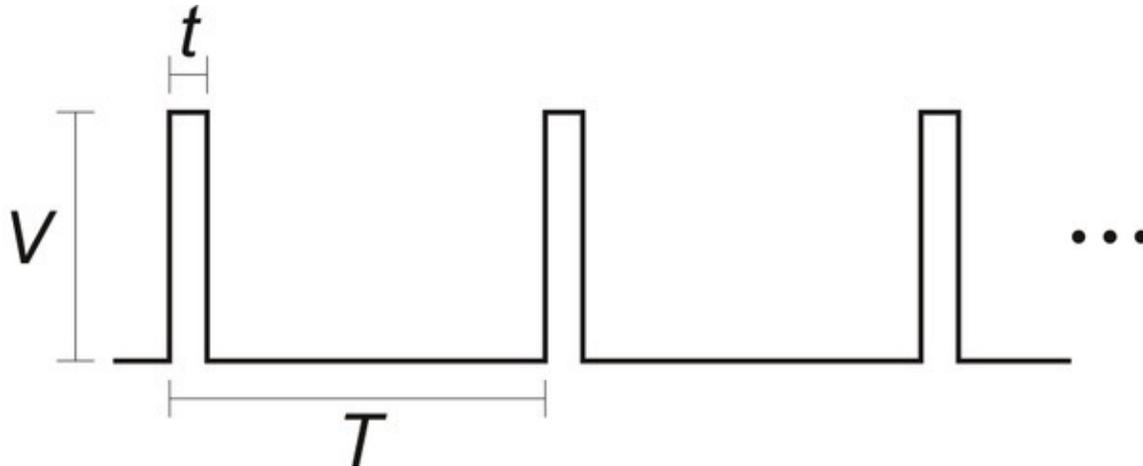
The signal should be low (0 V) normally and have periodic pulses with an amplitude ( $V$ ) of at least 2 V. The width of the pulses ( $t$ ) should be between 200  $\mu\text{s}$  and 2700  $\mu\text{s}$ . The period of the signal ( $T$ ), should be at most 100 ms, and there is no particular lower limit. When the Tic has received three good pulses in a row, it writes the width of the latest pulse to the “RC pulse width” variable in units of 1/12  $\mu\text{s}$ .
