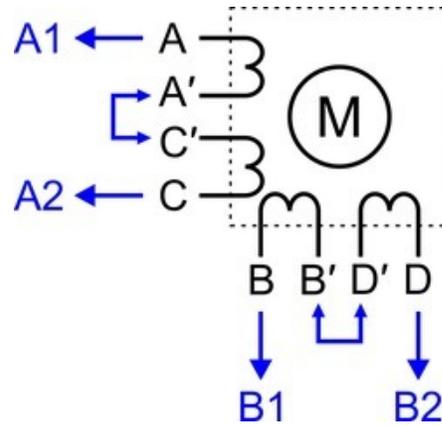
Connecting a two-phase unipolar/
