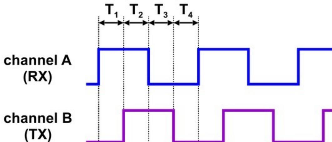
The time between the channel transitions (labeled  $T_{1-4}$  in the diagram above) must be at least 100  $\mu\text{s}$ . The signal must rise to 4 V or higher, and must stay within 0 V to 5 V.
