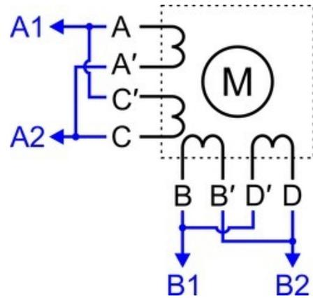
Connecting a two-phase unipolar/
