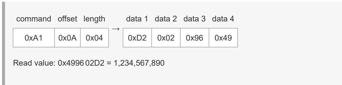
Starting with firmware version 1.07, you can set bit 6 of the length byte in order to add 128 to the offset without affecting the length. This allows you to access offsets between 128 and 255, which were previously inaccessible because the offset byte—like any data byte—must be between 0 and 127. In other words, bit 6 of the length byte is now treated as bit 7 of the desired offset, instead of bit 6 of the desired length.
