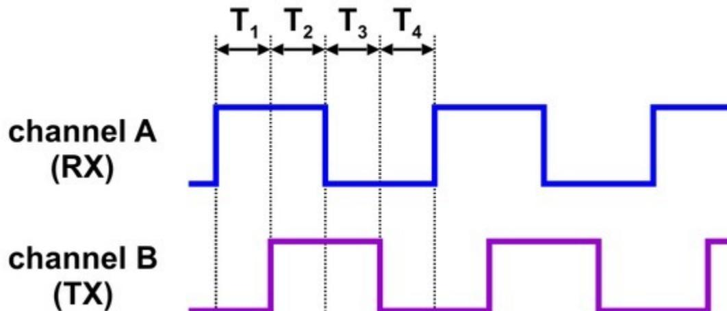
The time between the channel transitions (labeled T<sub>1-4</sub> in the diagram above) must be at least 100  $\mu$ s.
