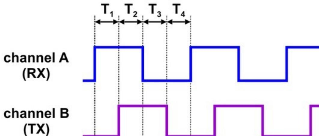
The time between the channel transitions (labeled  $T_{1-4}$  in the diagram above) must be at least 100  $\mu$ s.
