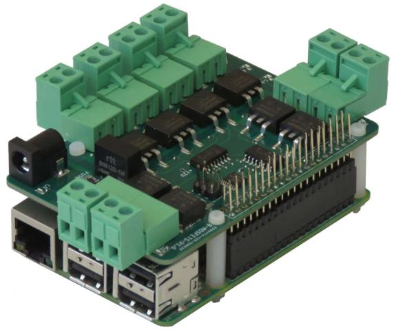
The 8-MOSFETS card is a stackable expansion card for Raspberry Pi. The card is compatible with all Raspberry Pi versions from Zero to 4. It offers a compact and inexpensive solution for adding up to 64 MOSFETs to your Raspberry Pi project.
