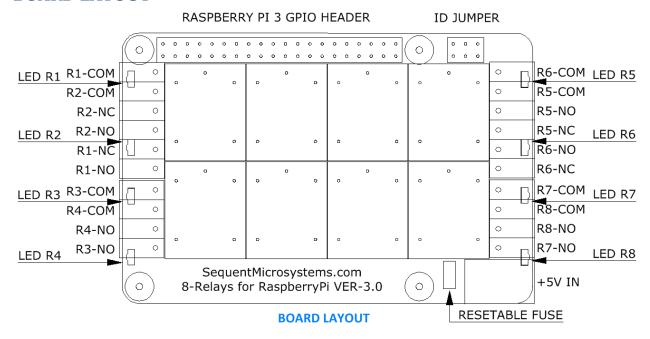
Your 8-RELAYS card comes with appropriate mounting hardware. Up to eight 8-RELAYS cards can be stacked on top of one Raspberry Pi.
