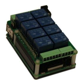
The 8-RELAYS card is a stackable expansion card for Raspberry Pi. The 8-RELAYS is compatible with all Raspberry Pi versions from Zero to 4. It offers a compact and inexpensive solution for adding up to 64 relays to your Raspberry Pi project.
