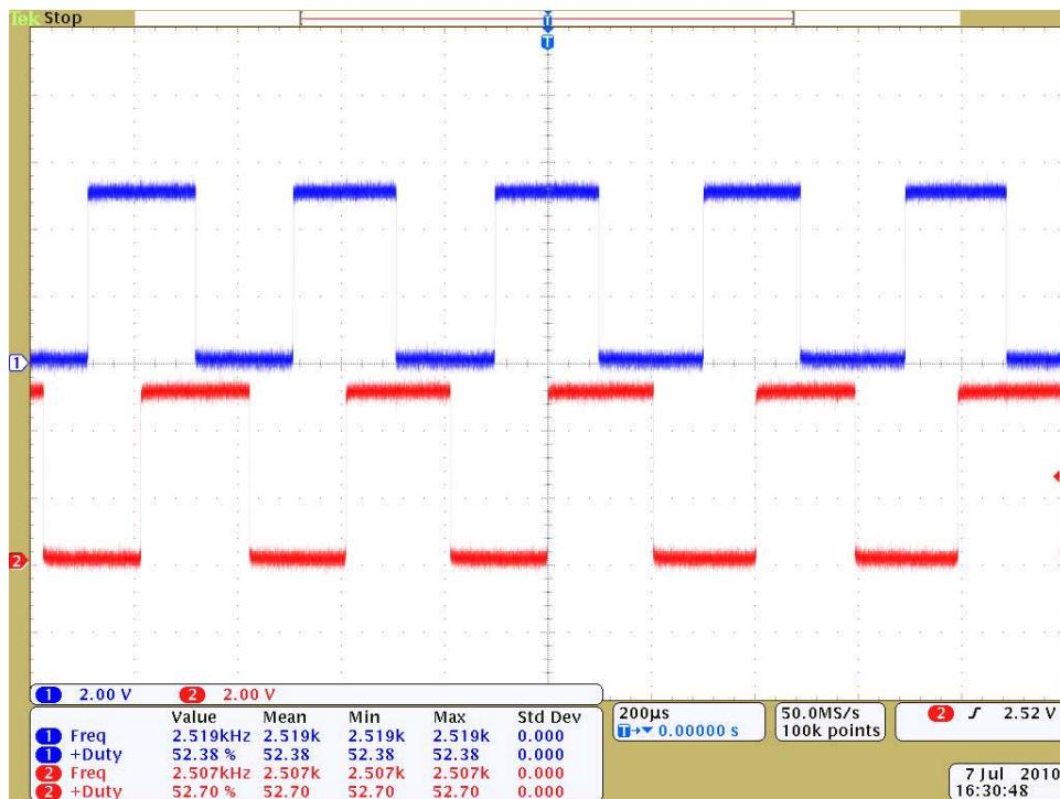
Counting both the rising and falling edges of both the A and B outputs results in 64 counts per revolution of the motor shaft. Using just a single edge of one channel results in 16 counts per revolution of the motor shaft, so the frequency of the A output in the above oscilloscope capture is 16 times the motor rotation frequency.
