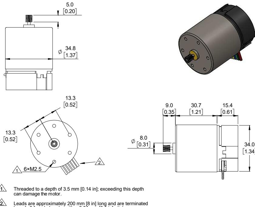
**1.** Threaded to a depth of 3.5 mm [0.14 in]; exceeding this depth can damage the motor.
