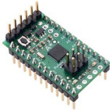
**A-Star 328PB Micro with included header pins soldered for breadboard use.**
