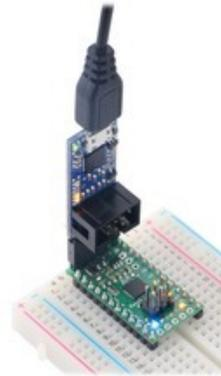
**A-Star 328PB Micro connected to the serial pins of a Pololu USB AVR Programmer v2.1.**
