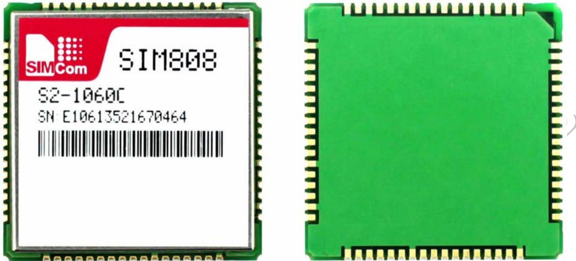
Figure 53: Top and Bottom View of SIM808
