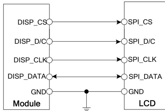
**Figure 39: LCD reference circuit**
