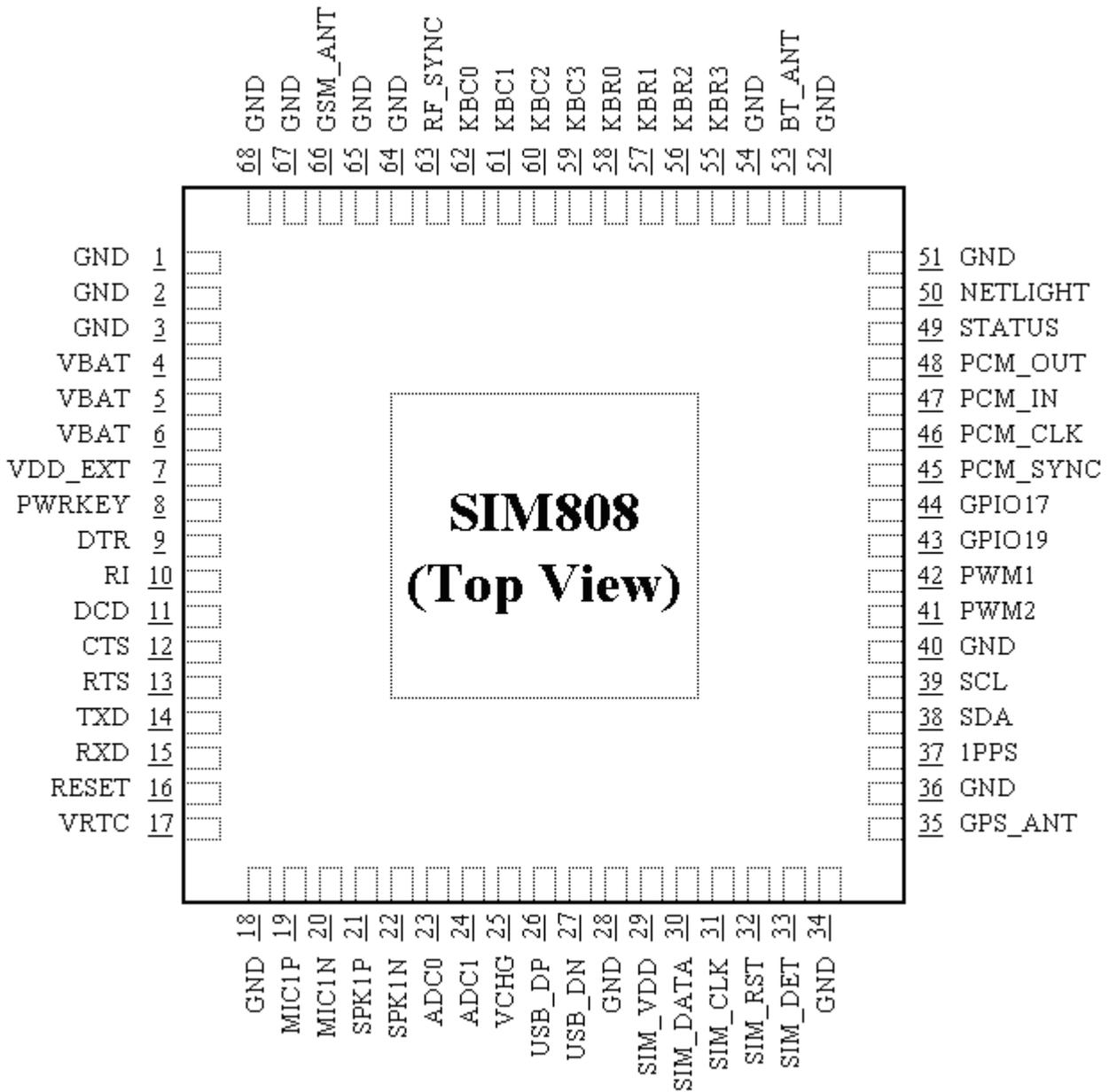
Figure 2: SIM808 pin out diagram (Top view)
