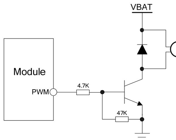
**Figure 44: Reference circuit of PWM drive buzzer**
