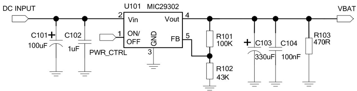
**Figure 6: Reference circuit of the LDO power supply**
