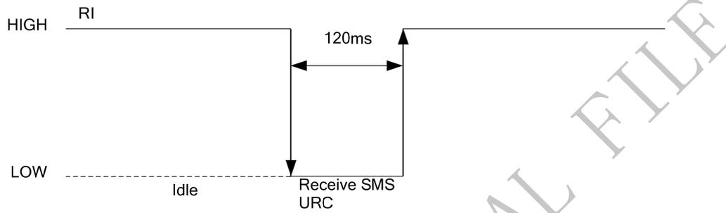
**Figure 29: RI behaviour of URC or receive SMS**
