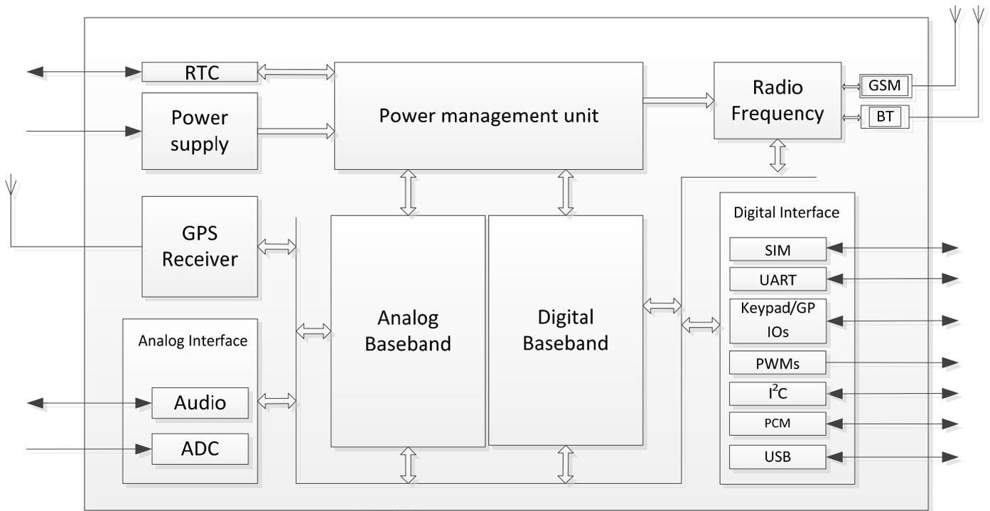
Figure 1: SIM808 functional diagram
