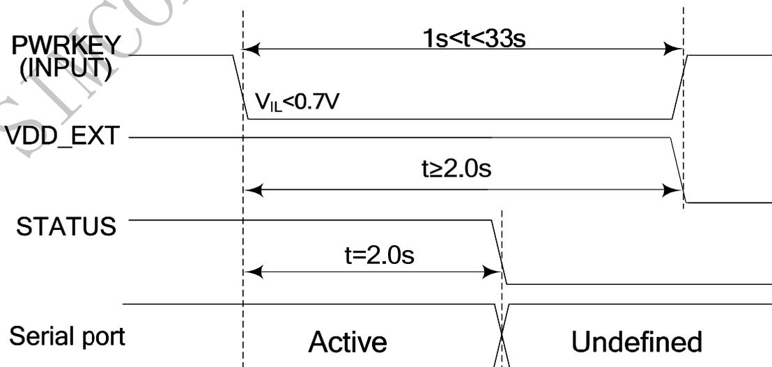
Figure 14: Timing of power off SIM808 by PWRKEY
