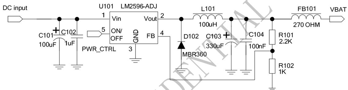
**Figure 7: Reference circuit of the DC-DC power supply**
