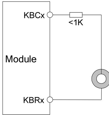
Figure 42: Enhance the ESD performance of keypad circuit
