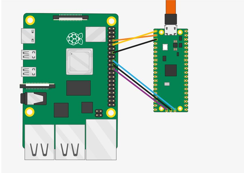
If possible you should wire the SWD port directly to the Raspberry Pi as signal integrity is important; wiring the SWD port via a breadboard or other indirect methods may reduce the signal integrity sufficiently so that loading code over the connection is erratic or fails completely. It is important to also wire the ground wire (0v) between the two directly and not rely on another ground path.
