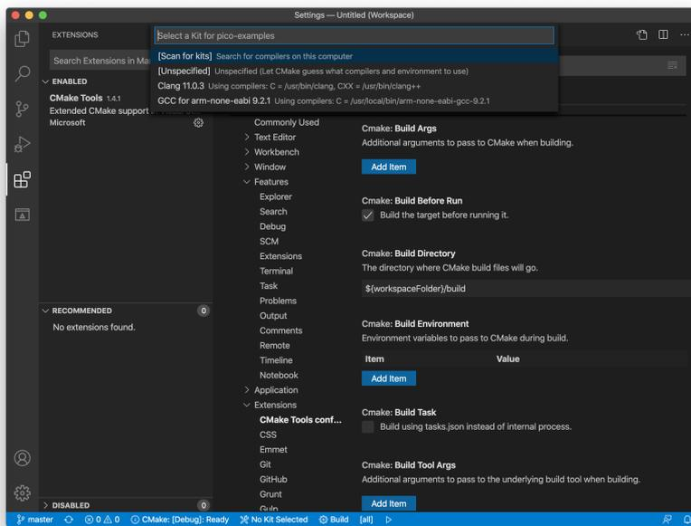
Finally go ahead and click on the "Build" button (with a cog wheel) in the blue bottom bar of the window. This will create the build directory and run CMake as we did by hand in [Section 3.1](#), before starting the build itself, see [Figure 8](#).
