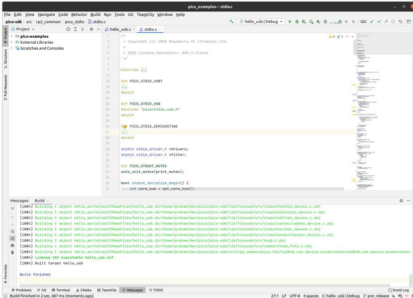
Note that the drop down selector lets you choose both the target you want to build and a CMake profile to use (in this case one of `Debug` or `Release`)
