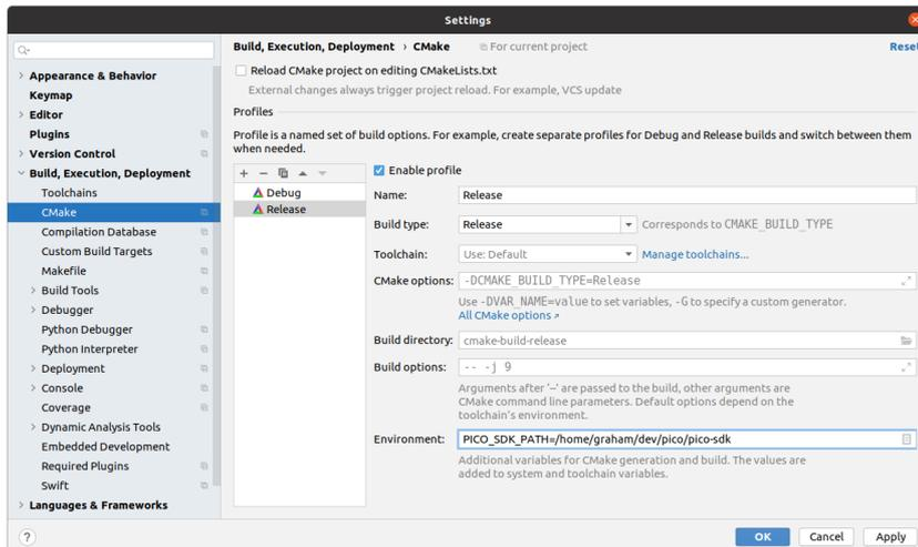
After pressing OK, you'll see something like Figure 30. Note that there are two tabs for the two profiles (**Debug** and **Release**) at the bottom of the window. In this case **Release** is selected, and you can see that the CMake setup was successful.
