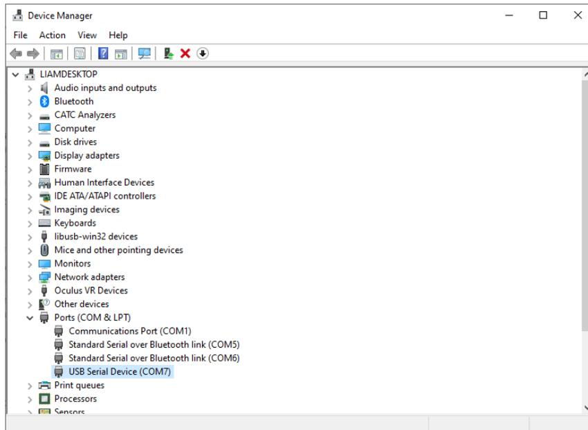
Open PuTTY. Select **Serial** under connection type. Then type the name of your COM port along with 115200 as the speed.
