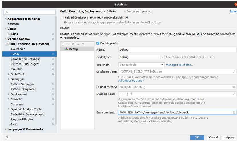
You can have as many CMake profiles as you like with different settings. You probably want to add a **Release** build by hitting the **+** button, and then filling in the `PICO_SDK_PATH` again, or by hitting the copy button two to the right, and fixing the name and settings (see Figure 29)
