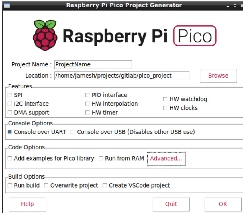
You can add specific features to your project by selecting them from the check boxes on the GUI. This will ensure the build system adds the appropriate code to the build, and also adds simple example code to the project showing how to use the feature.
