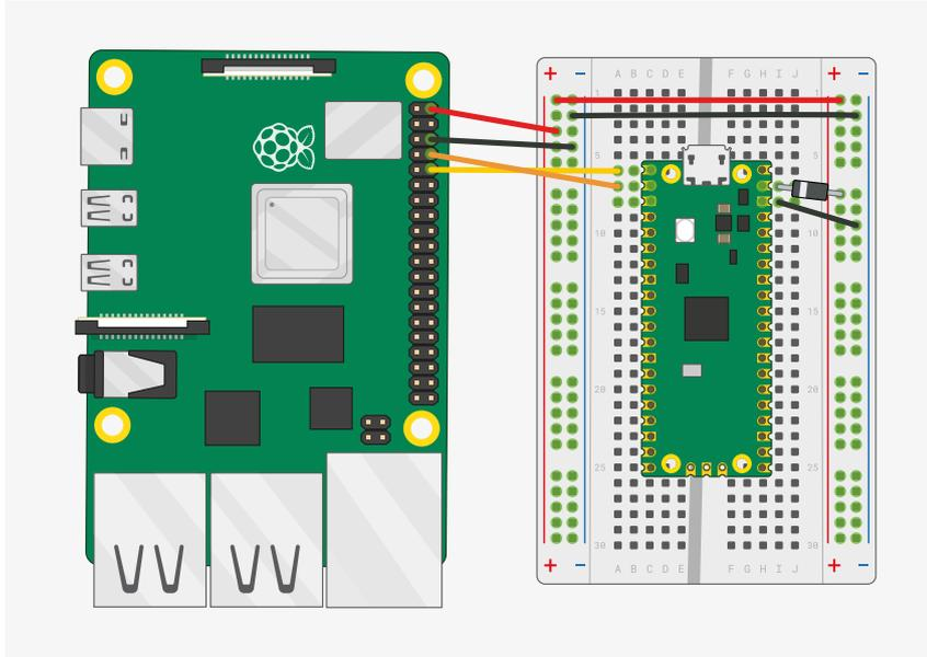
Whilst it is possible to connect the Raspberry Pi's 5V pin to the Raspberry Pi Pico VBUS pin, this is not recommended. Shorting the 5V rails together will mean that the Micro USB cannot be used. An exception is when using the Raspberry Pi Pico in USB host mode, in this case 5V must be connected to the VBUS pin.
