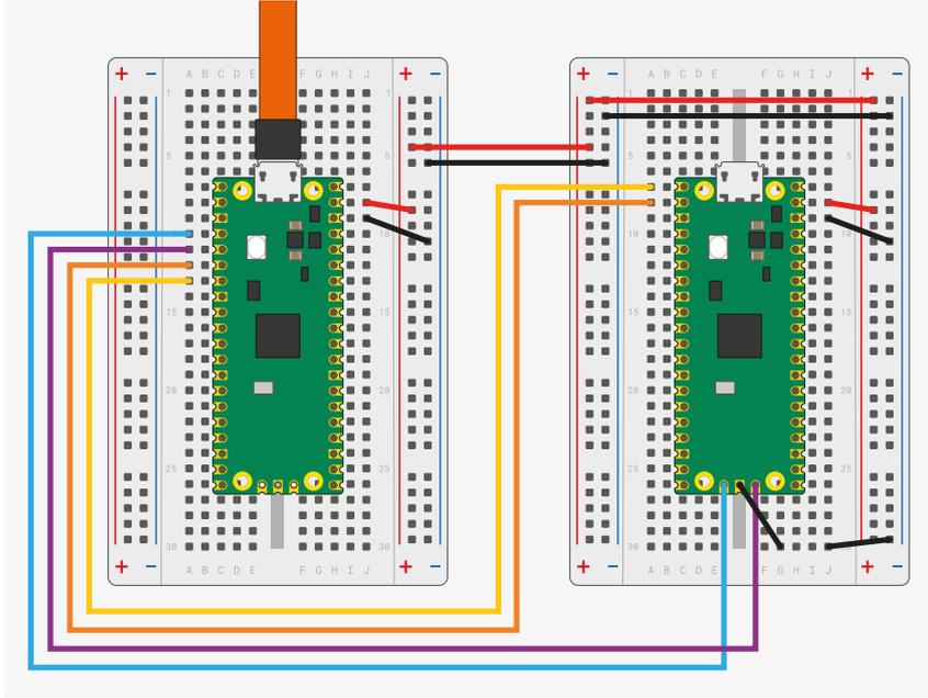
The wiring loom between the two Pico boards is shown in [Figure 34](#).
