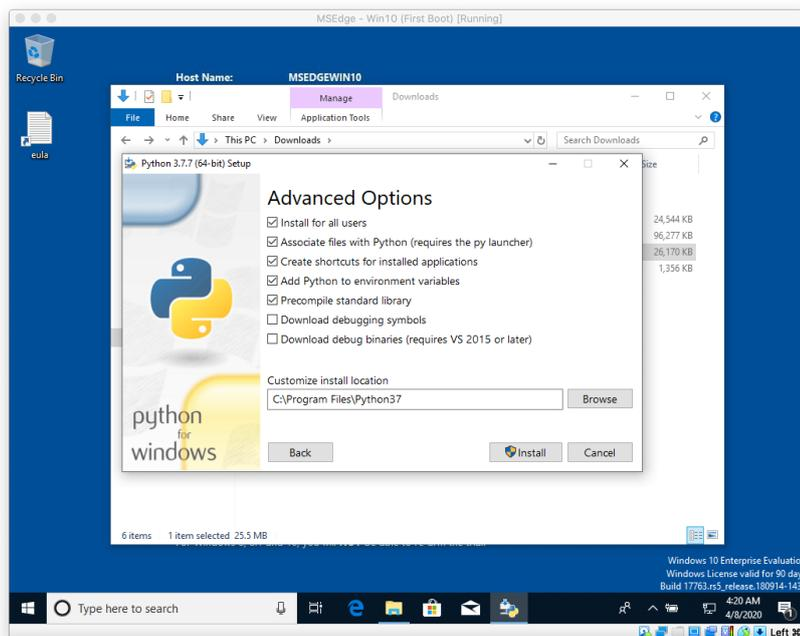
Additionally, when installing Python chose 'Customize installation,' click through 'Optional Features' and then under 'Advanced Features' choose to 'Install for all users'.
