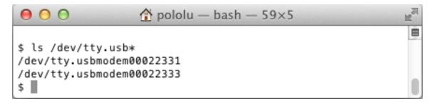
The entry with the **lowest number** is the programming port, and later you will need to pass its name as a parameter to AVRDUDE.
