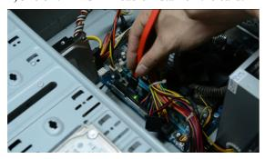
5) SATA HDD contact 15pin power cable from PC
