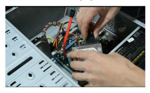
6) Other of 7PIN cable install on the SATA HDD
