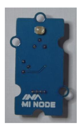
ModuleConnect TypeAvailable ConnectorsLight SensorAnalogA0, A1, A2
