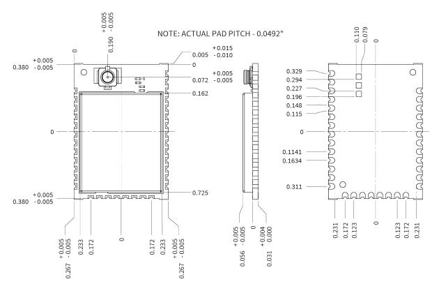
Mechanical drawings XBee 3 micro antennas
