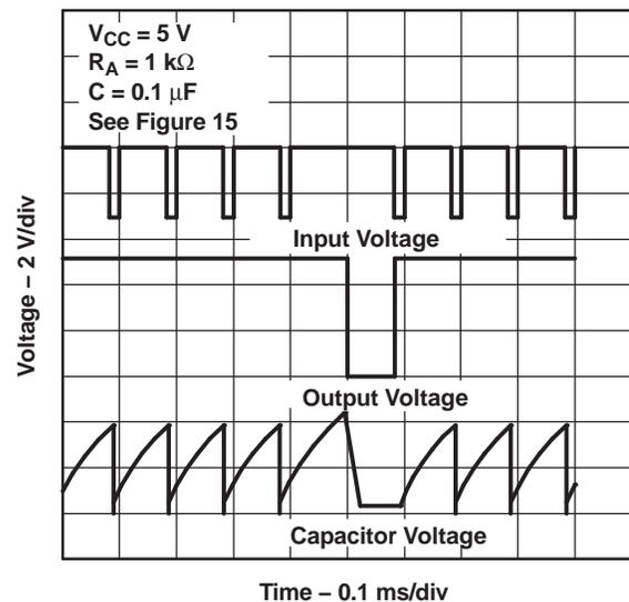
Figure 16. Completed Timing Waveforms for Missing-Pulse Detector
