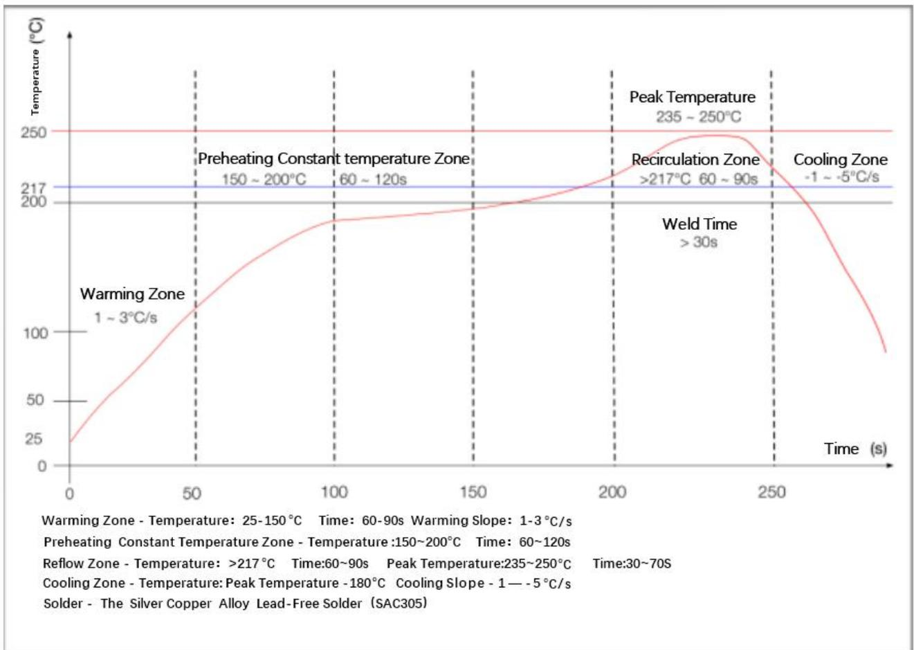
Figure 17 Reflow welding curve
