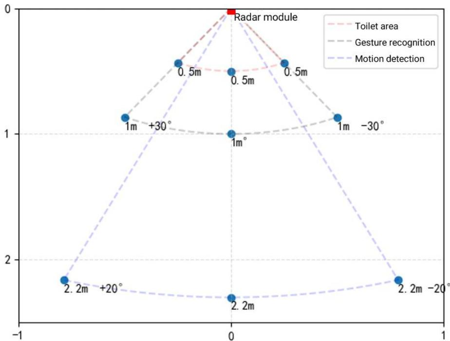
**Figure 14 Gesture recognition hanging wall radar power diagram**
