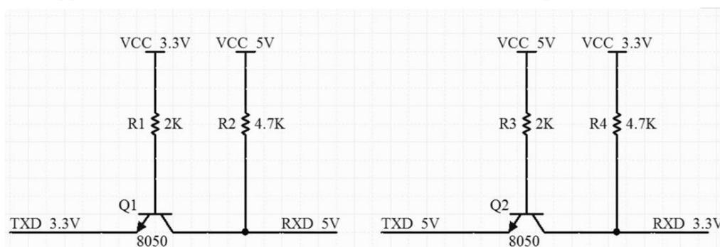
Figure 16 Level switching circuit
