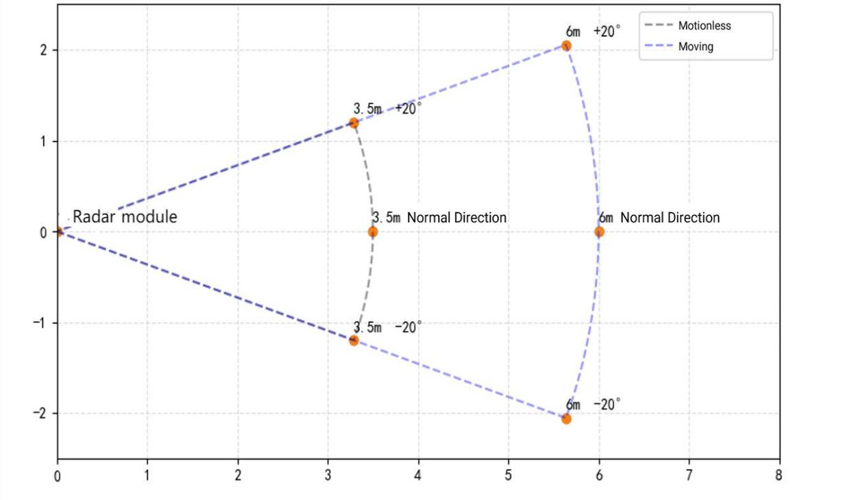
**Figure 11 Power map of precision ranging wall-mounted radar**
