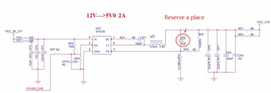
Figure 15 DC-DC step-down circuit diagram
