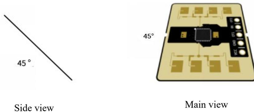
**Figure 12 Schematic diagram of tilted installation for gesture recognition**
