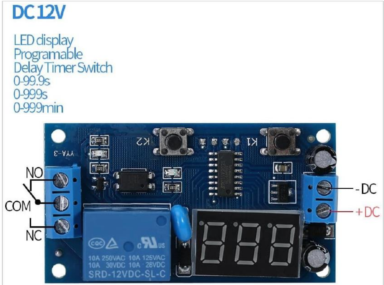
Image 5: DC 12V Programmable Delay Timer Switch. This image highlights the NO (Normally Open), COM (Common), and NC (Normally Closed) terminals of the relay, along with the DC 12V power input terminals. The LED display indicates the current state and timing.
