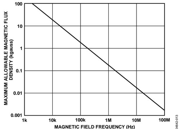
Figure 13. Maximum Allowable External Magnetic Flux Density
