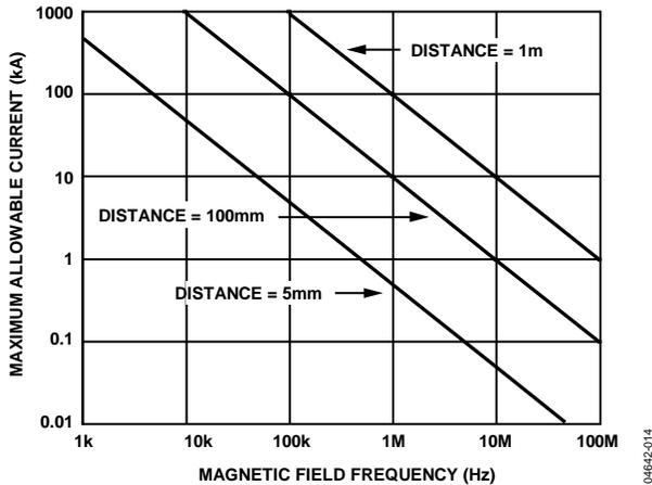
Figure 14. Maximum Allowable Current for Various Current-to-ADuM1200/ADuM1201 Spacings
