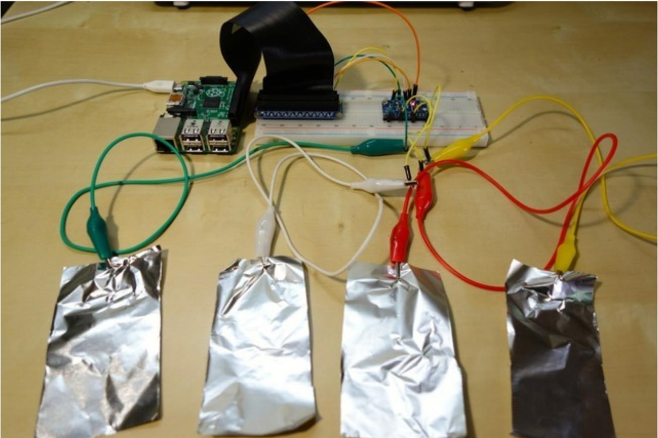
Reach out and touch someone, or *something*, with the MPR121 capacitive touch sensor and a Raspberry Pi or BeagleBone Black! This breakout provides 12 capacitive touch inputs and all the logic to read them over a simple I2C communication bus. For example you can make your own buttons, detect if someone touched a device, create a fun [plush game controller \(http://adafru.it/ne8\)](http://adafru.it/ne8), or even a wacky devices like a [banana piano \(http://adafru.it/eid\)](http://adafru.it/eid)!
