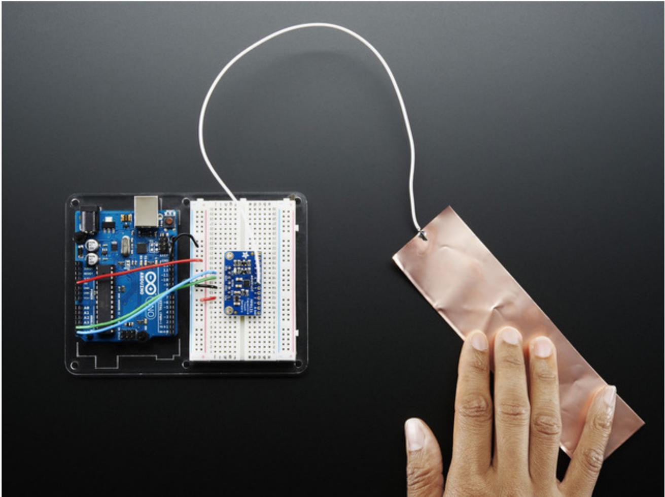
Once you have the MPR121 breakout working you'll want to construct electrodes. These are large conductive piece of copper, foil, paint, etc that will act as the "thing you touch"
