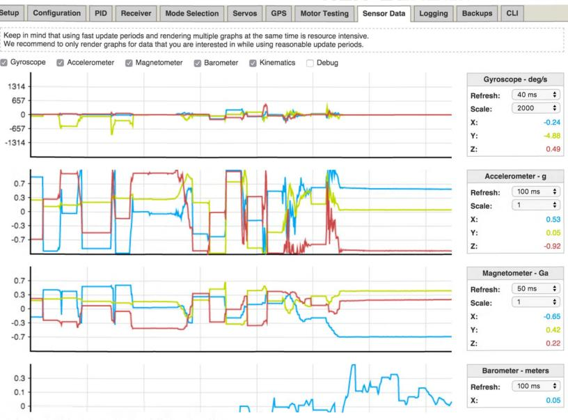
You should use the raw sensor data page to check your sensors. When moving the board, you should see movement on the accelerometer, gyro, magnetometer, barometer, etc.
