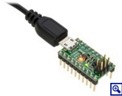
Printed on the A\* circuit board are indicators that you can use to quickly identify each pin's capabilities: a triangle next to the pin means it can be used as an analog input, and a square wave symbol under the pin number means it can be used as a PWM output.
