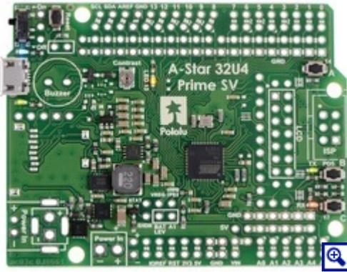
The **A-Star 32U4 Prime SV** can be powered from a **5 V to 36 V** external source. The input voltage is regulated to 5 V by a 1 A ISL85410 switching step-down (buck) converter from Intersil. (We also make a **standalone regulator** [<https://www.pololu.com/product/2831>] based on this integrated circuit.)
