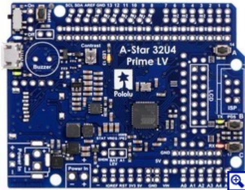
The **A-Star 32U4 Prime LV** can be powered from a **2.7 V to 11.8 V** external source. The input voltage is regulated to 5 V by a TPS63061 switching step-up/step-down (buck-boost) converter from Texas Instruments. (We also make a **standalone regulator** [<https://www.pololu.com/product/2123>] based on this integrated circuit.)
