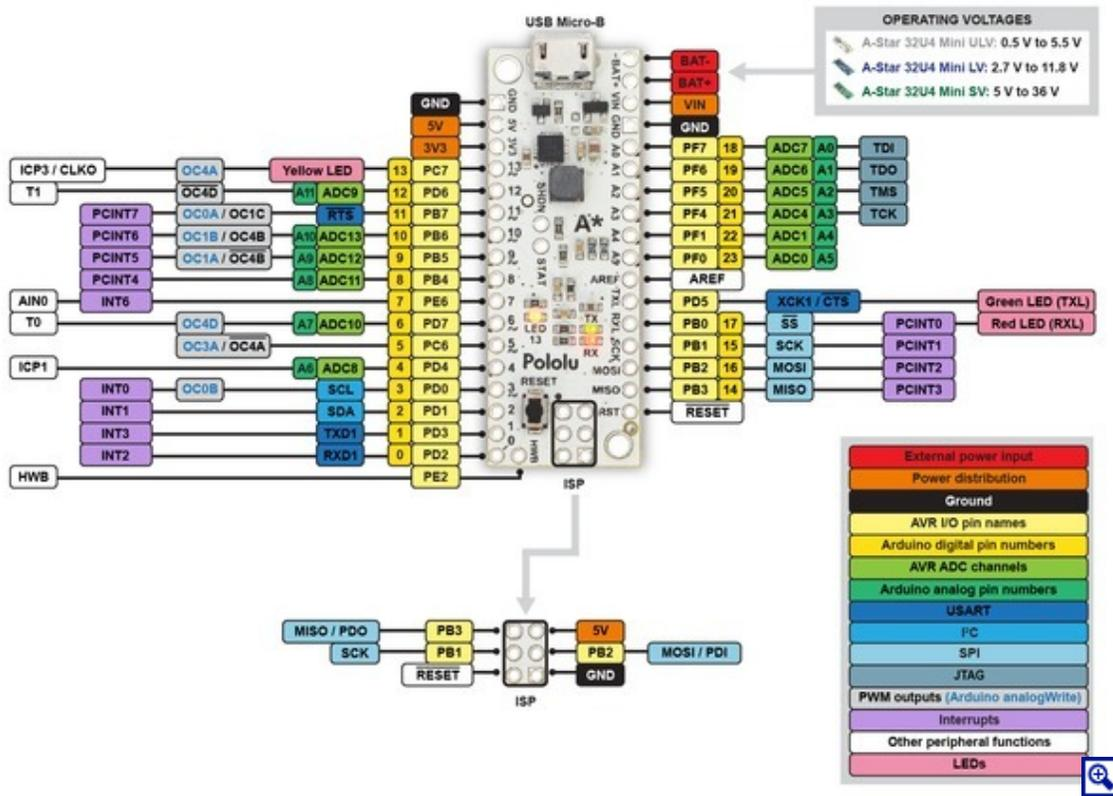
This diagram identifies the I/O and power pins on the A-Star 32U4 Mini (ULV, LV, and SV versions); it is also available as a **printable PDF** [[https://www.pololu.com/file/download/a-star-32u4-mini-pinout.pdf?file\\_id=0J784](https://www.pololu.com/file/download/a-star-32u4-mini-pinout.pdf?file_id=0J784)] (269k pdf). For more information about the ATmega32U4 microcontroller and its peripherals, see Atmel's ATmega32U4 documentation.
