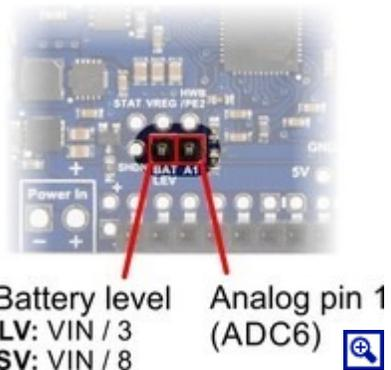
Battery level Analog pin 1 (ADC6) jumper on the A-Star 32U4 Prime.
