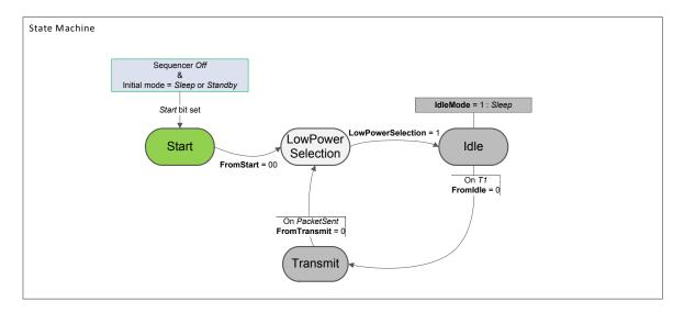
Figure 53. Beacon Mode State Machine
