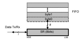
Figure 26. FIFO and Shift Register (SR)
