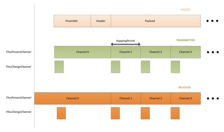
Figure 7. Interrupts Generated in the Case of Successful Frequency Hopping Communication.
