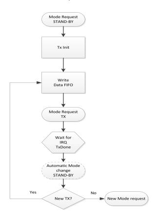
Figure 9. LoRa<sup>TM</sup> Modulation Transmission Sequence.
