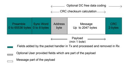
Figure 33. Fixed Length Packet Format
