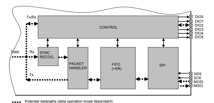
Figure 25. SX1276/77/78/79 Data Processing Conceptual View
