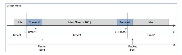
Figure 52. Beacon Mode Timing Diagram
