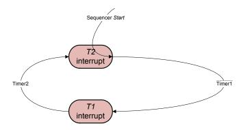
Figure 23. Timer1 and Timer2 Mechanism
