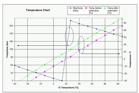
Figure 41. Temperature Sensor Response
