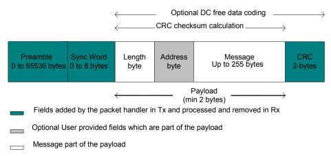
Figure 34. Variable Length Packet Format
