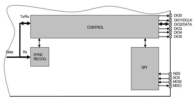
Figure 29. Continuous Mode Conceptual View
