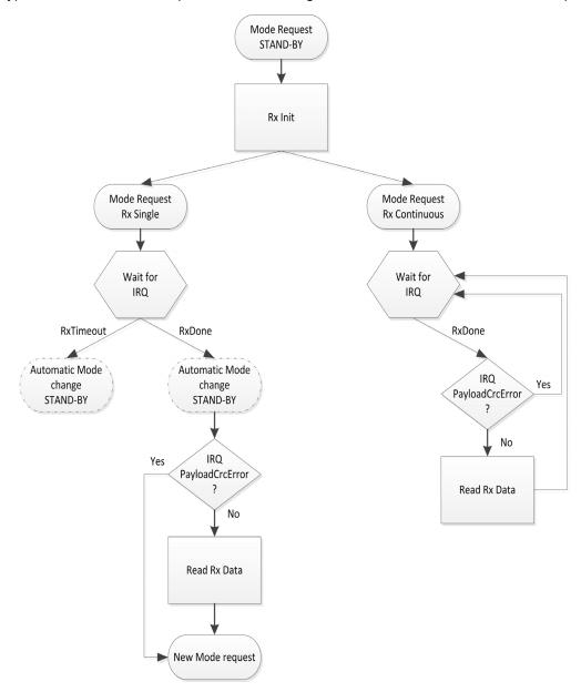
Figure 10. LoRa<sup>TM</sup> Receive Sequence.
