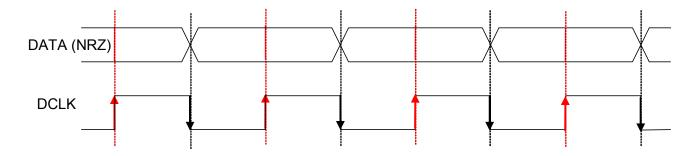
Figure 31. Rx Processing in Continuous Mode
