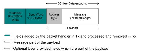
Figure 35. Unlimited Length Packet Format
