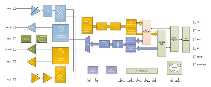
Figure 4. SX1276/77/78/79 Block Schematic Diagram
