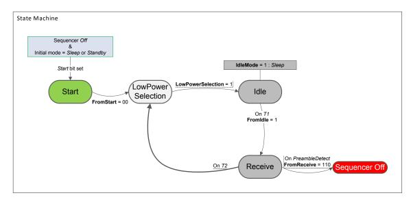
Figure 47. Wake On PreambleDetect State Machine
