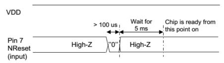
Figure 43. Manual Reset Timing Diagram
