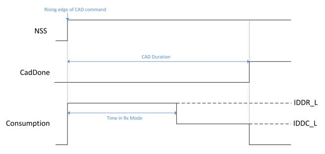
Figure 13. Consumption Profile of the LoRa CAD Process
