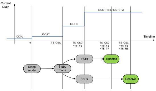
Figure 17. Startup Process
