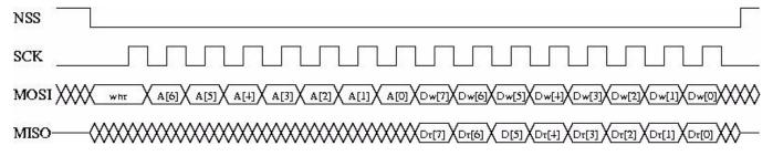
Figure 38. SPI Timing Diagram (single access)
