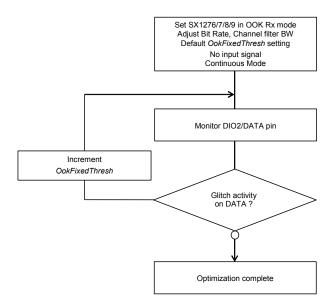
Figure 15. Floor Threshold Optimization
