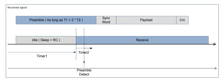
Figure 46. Listen Mode with Preamble Received
