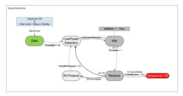
Figure 51. Wake On SyncAddress State Machine
