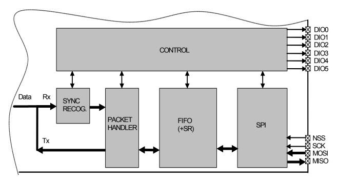
Figure 32. Packet Mode Conceptual View
