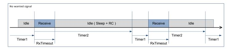
Figure 48. Listen Mode with no SyncAddress Detected
