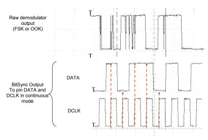
Figure 16. Bit Synchronizer Description
