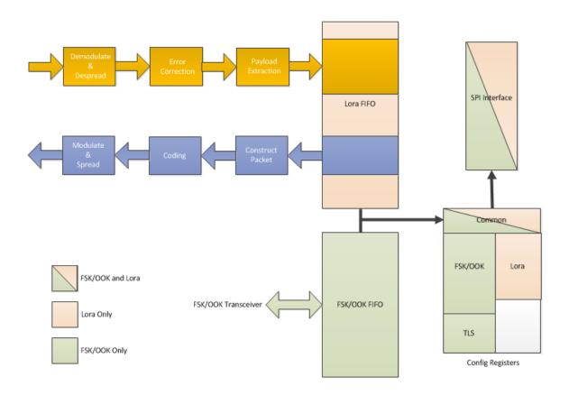
Figure 5. LoRa<sup>TM</sup> Modem Connectivity
