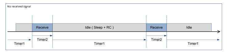
Figure 45. Listen Mode with No Preamble Received
