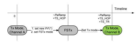
Figure 22. Transmitter Hopping
