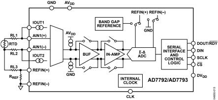
Figure 21. RTD Application Using the AD7792/AD7793
