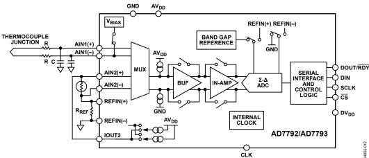
Figure 20. Thermocouple Measurement Using the AD7792/AD7793
