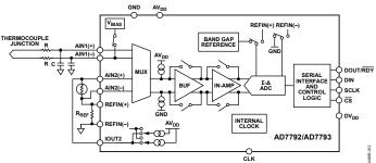
Figure 12. Basic Connection Diagram
