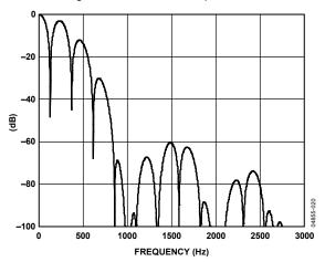
Figure 15. Filter Profile with Update Rate = 242 Hz
