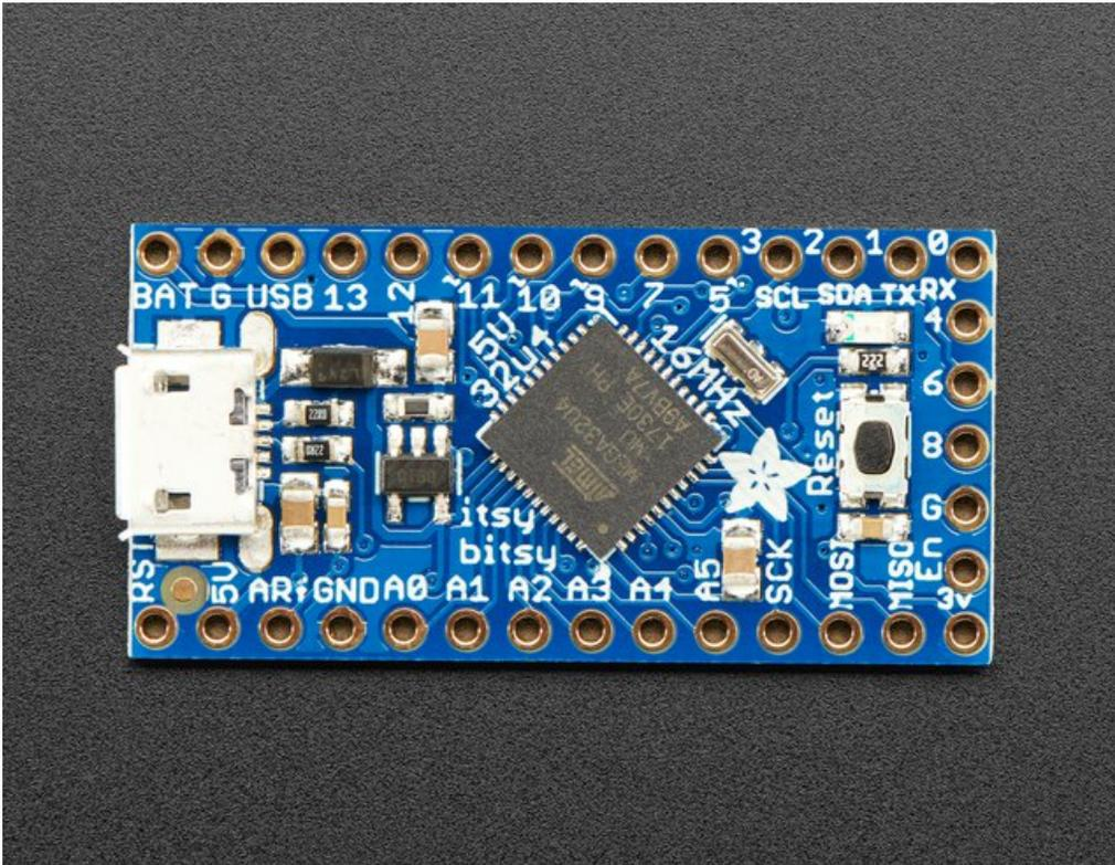
The **Itsy Bitsy 32u4** uses the ATmega32u4 chip, which is the same core chip in the Arduino Leonardo as well as the same chip we use in our Feather 32u4. The **5V 16 MHz** It runs at the same speed and voltage of an Arduino UNO or Leonardo. The **3V 8 MHz** version is the same speed and voltage as a Feather 32u4. So you'll be happy to hear that not only is Itsy Bitsy programmable using the Arduino IDE as you already set up, but a vast number of Arduino projects will work out of the box!
