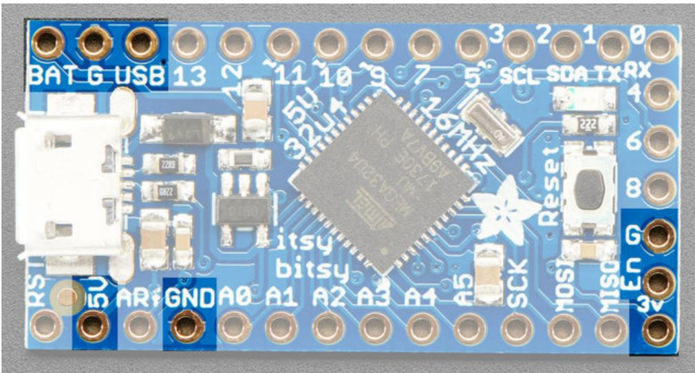
In addition to the three standard power pins, the 5V ItsyBitsy has a few more pins available for power sourcing:
