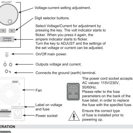
Please refer to the fuse parameters on the back of the fuse label, in order to replace the fuse with the specifed fuse.
