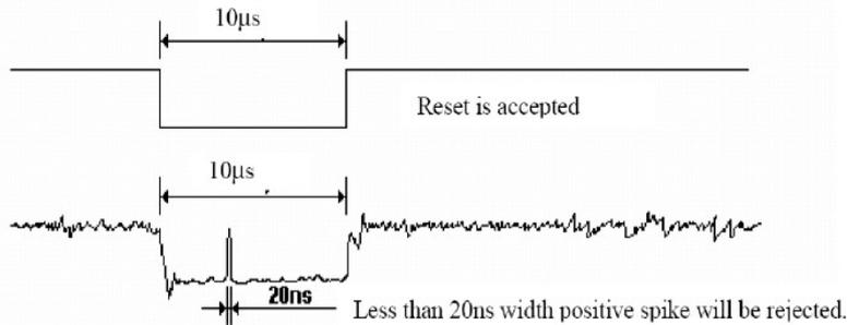
5. It is necessary to wait 5msec after releasing RESX before sending commands. Also Sleep Out command cannot be sent for 120msec.
