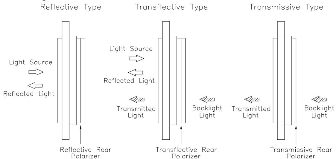
**10. Electro-Optical Characteristics Test Method**
