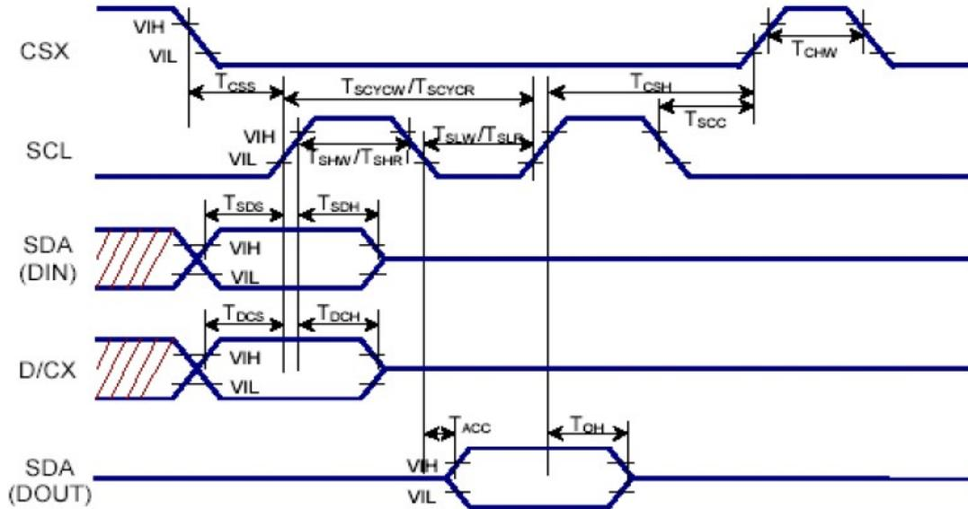
**Table 17.3.2.2: 4 pin Serial Interface Characteristics**
