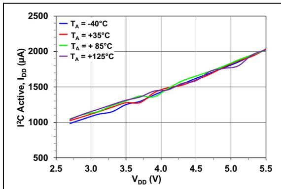
**FIGURE 2-26:**  $I^2C$  Active,  $I_{DD}$  Across  $V_{DD}$ .
