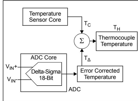
**FIGURE 5-2:** Thermocouple Temperature Register Block Diagram.
