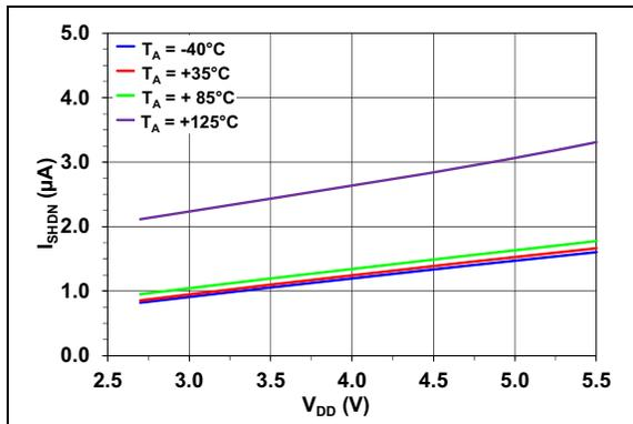
**FIGURE 2-27:** Shutdown Current,  $I_{SHDN}$  Across  $V_{DD}$ .
