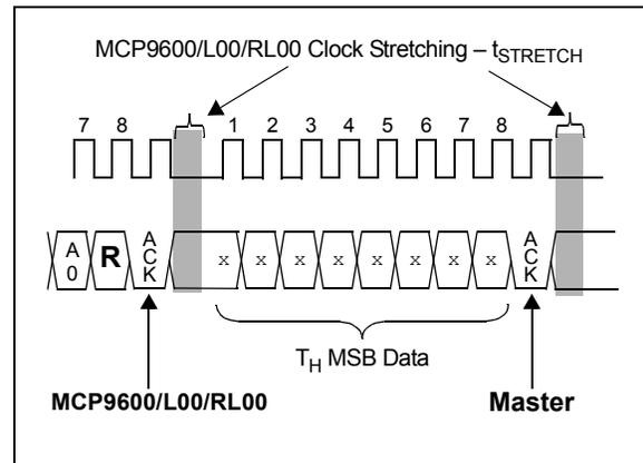
**FIGURE 4-2:** Clock Stretching.
