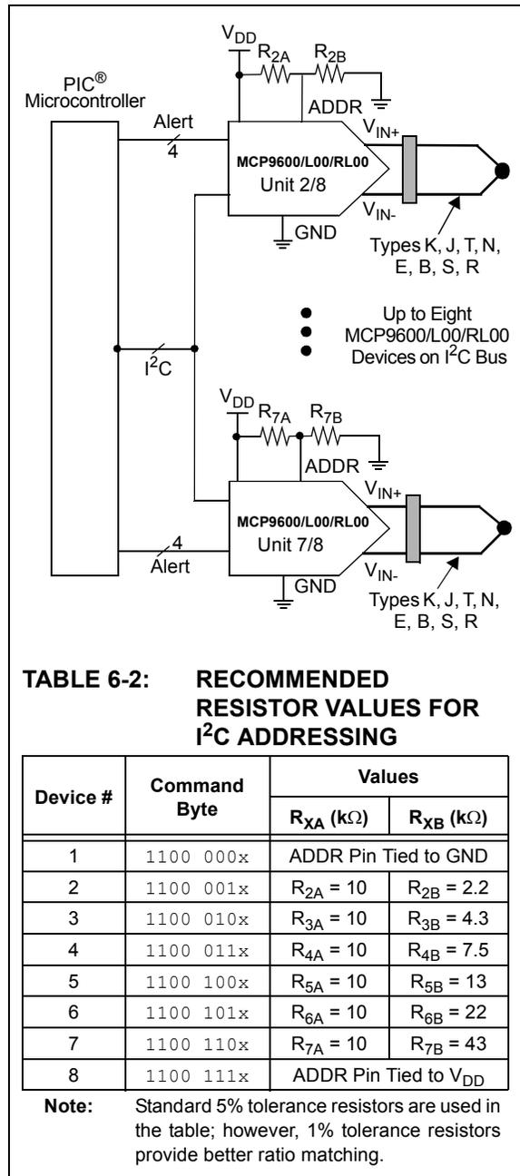
**FIGURE 6-4:** I<sup>2</sup>C Address Selection Implementation.
