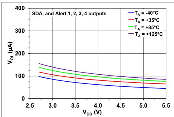
**FIGURE 2-21:** SDA and Alert Outputs,  $V_{OL}$  Across  $V_{DD}$ .
