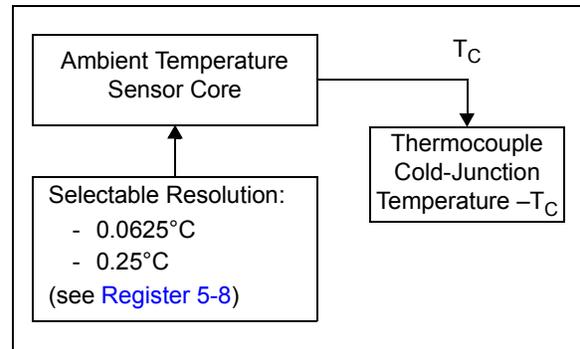
**FIGURE 5-4: Thermocouple Cold-Junction Register (T<sub>C</sub>) Block Diagram.**
