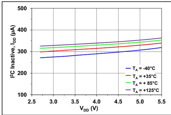
**FIGURE 2-25:**  $I^2C$  Inactive,  $I_{DD}$  Across  $V_{DD}$ .
