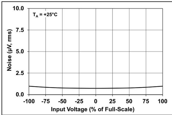
**FIGURE 2-19:** Input Noise, % of Full Scale.
