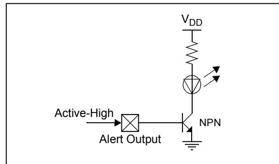
**FIGURE 6-3:** Alert Output Buffer for LED Indicator.
