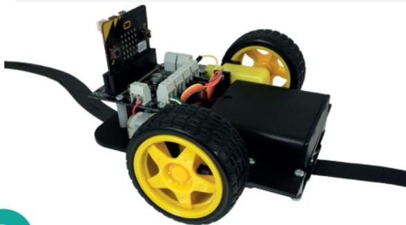
**NOTE:** The buggy can be programmed to work with a dark coloured line on a light background or a light coloured line on a darker background!
