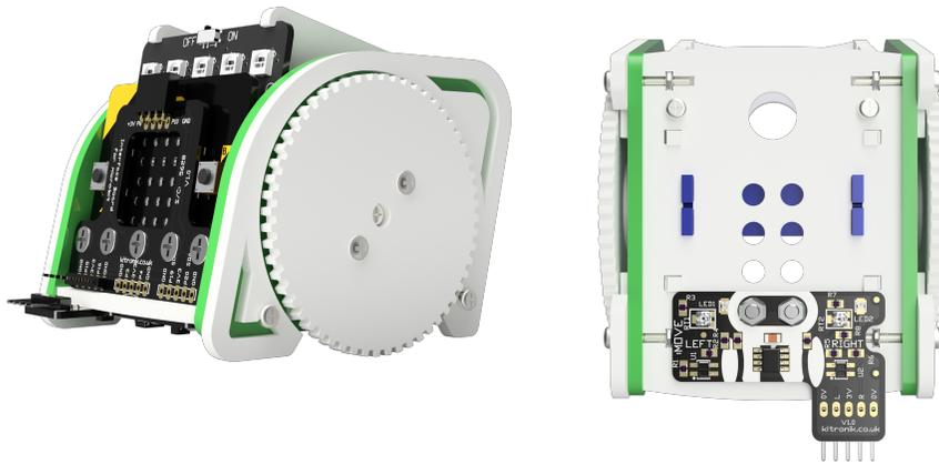
**Examples of board in use:** This breakout board can be used with our :MOVE mini robot. For more details see: [www.kitronik.co.uk/movemini](http://www.kitronik.co.uk/movemini)
