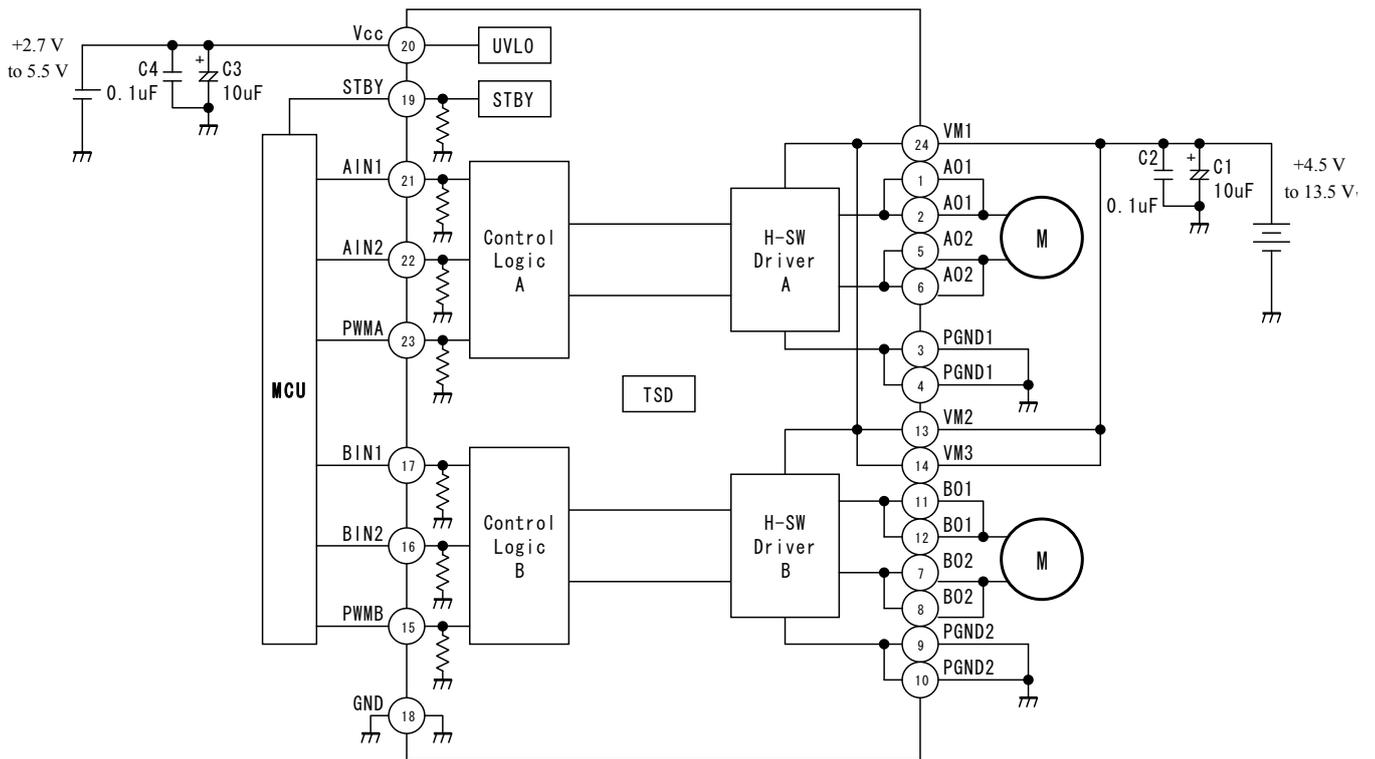
Note: Condensers for noise absorption (C1, C2, C3, and C4) should be connected as close as possible to the IC.
